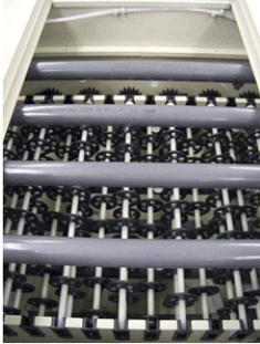
All 2300 systems feature oscillating top and bottom spray tubes in the main etching and developing sections. Each tube can have up to four nozzles. Different types of nozzles and flow rates are available to optimize the performance for the application. The standard conveyor features large elastomer wheels for reliable transport. Thin material conveyor options for transporting material as thin as 25 microns are also available.
