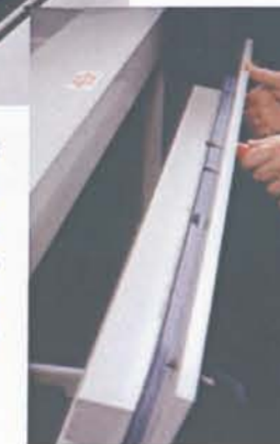
Developer, etcher, and stripper lids and doors are sealed with Chemcut's patented air seals for solution and fume containment
