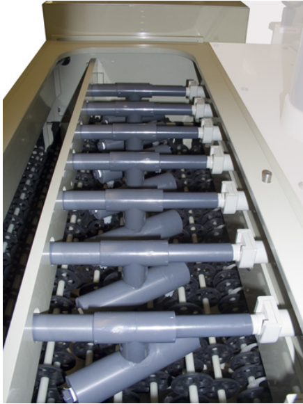
Inside the EAM showing seven of the top side spray zones. (30 Inch Wide System)
