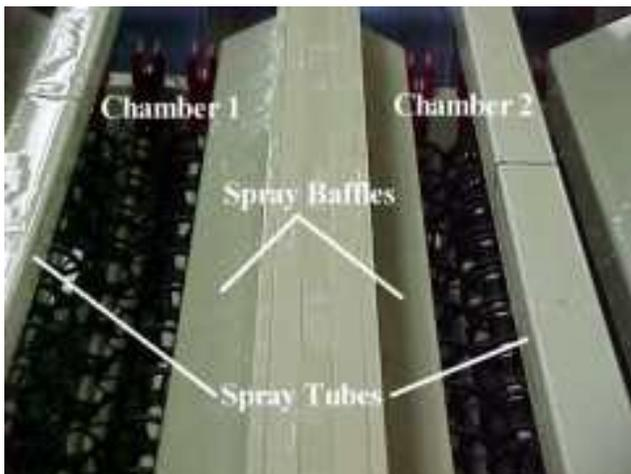
Chamber Transition with Spray Baffles in Place
