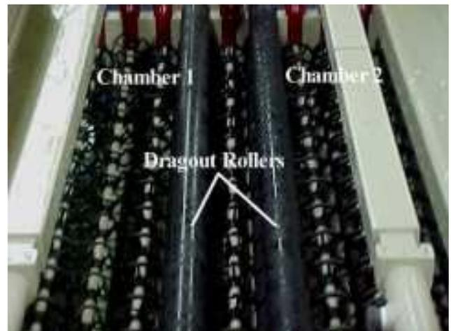
Chamber Transition with Baffles removed
